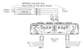
The use of twisted pair interconnects is recommended for all installations to minimize noise. When routing these cables through the automobile, try to keep them away from factory wiring harnesses and other power wiring. If you need to cross any of this wiring do so at a 90 degree angle to reduce the potential of noise problems.
